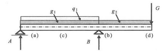
Figure 5: Beam with overhangs - a decisive combination for determining the extreme bending momentum in the field (point c) (STR).  $\gamma_{g1}=1,35$ ,  $\gamma_{g2}=1,0$ ,  $\gamma_G=1,0$ ,  $\gamma_{q1}=1,5$ ,  $\gamma_{q2}=0,0$
