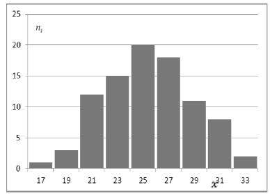
**Fig. A.1** Histogram of the grouped data form Example 3.9 (90 observations of concrete strength)
