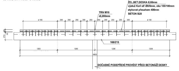
Figure 7 - beam- slab interconnection
