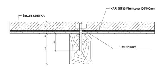
Figure 8 - beam- slab interconnection - section
