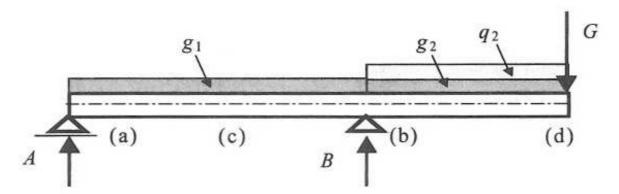
Figure 4: Beam with overhangs - a decisive combination for determining the static balance (reaction A) (EQU).  $\gamma_{g1}=0.9$ ,  $\gamma_{g2}=1.1$ ,  $\gamma_G=1.1$ ,  $\gamma_{q1}=0.0$ ,  $\gamma_{q2}=1.5$
