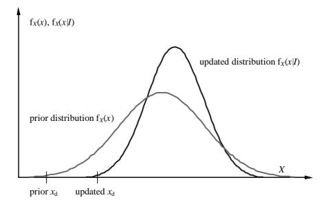
Figure 1: Updating of probability density function for an expected variable *X*.
