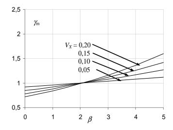
Fig. B.3. Variation of  $\gamma_m$  with  $\beta$  for selected coefficients of variation  $V_X$  and log-normal distribution of *X*.
