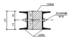
Figure 10 – beam steel liners - section
