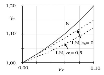
Fig. B.4. Variation of  $\gamma_m$  with  $\beta$  for selected coefficients of variation  $V_X$ , normal and log-normal distribution of X
