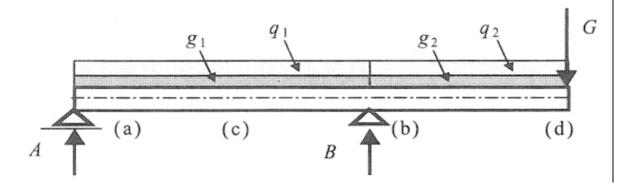
Figure 2: Beam with overhangs - assuming three independent permanent loads  $g_1,g_2,G$  and two independent variables loads  $q_1, q_2$ .
