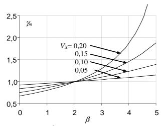
Fig. B.2. Variation of  $\gamma_m$  with  $\beta$  for selected coefficients of variation  $V_X$  and normal distribution of X
