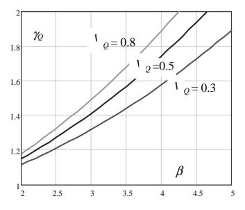
Fig. B.7. Variation of  $\gamma_Q$  with the reliability index  $\beta$  for selected values of the coefficients of variation  $V_Q$  assuming a Gumbel distribution of Q, period ratio N = 10 and  $\alpha_T = 1$
