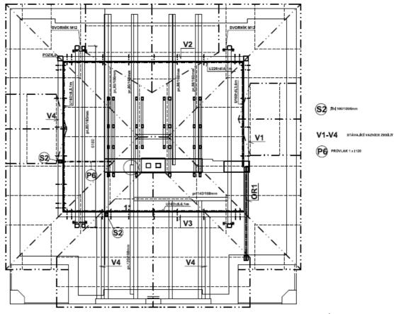
Figure 5 – proposed changes to the truss and ceiling above the 1<sup>st</sup> floor
